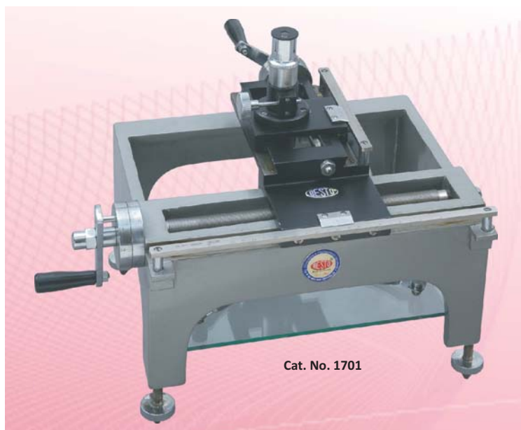
Special measuring microscope with least count of 0.0001cm.
